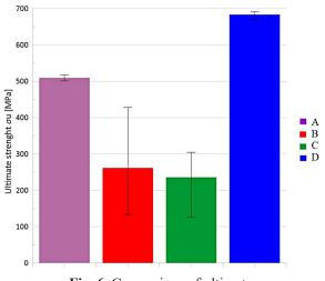
Fig. 6. Comparison of ultimate strength among specimen series
