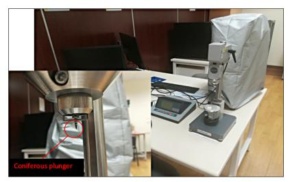
Fig. 1. Hardness-testing machine M SHORE D/C/D0 0.5 with a coniferous plunger
